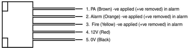
Figure 21. Communications Wiring Harness.
